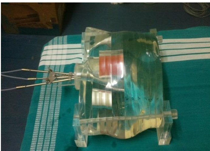
Fig 1:- The Indigenously Fabricated Female Pelvis Phantom in Treatment Position for EBRT and Brachytherapy
