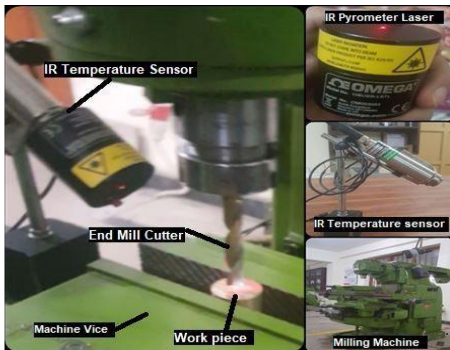
Fig 2:- Experimental Setup for Temperature Measurement
