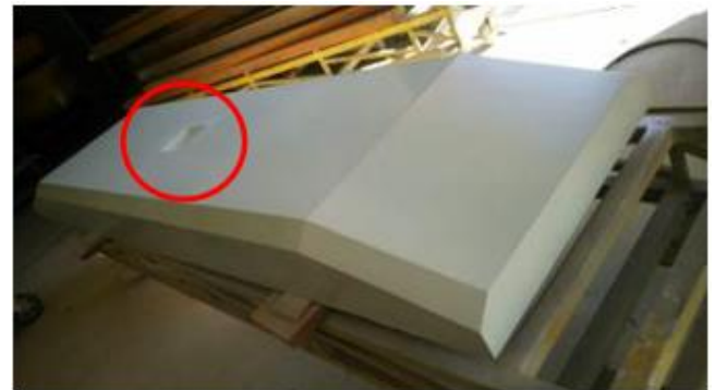
Fig 4:- Location of the hole where the dredging pipe is seen from the bottom of the model
