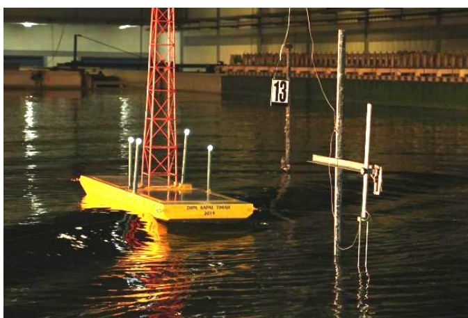
Fig 15:- Seakeeping Test on H_s = 2.5 m, T_p = 8.5 sec, Heading Angle = 135 deg
