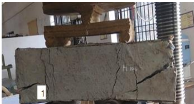
Fig 9:- Failure of the Headed Stud Beam
