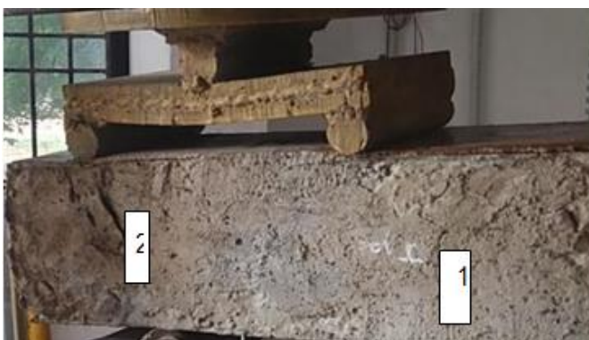
Fig 11:-Shaer Failure of the Beam at the Ultimate Stage
