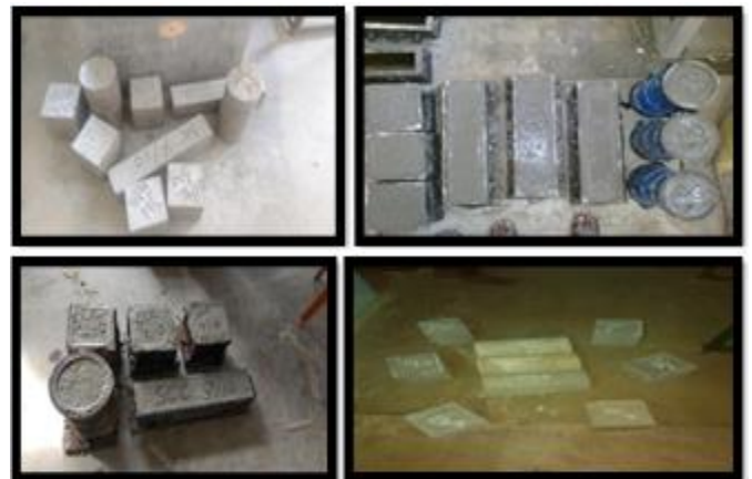
Fig 8:- The casting of various % SAP and CC specimen
