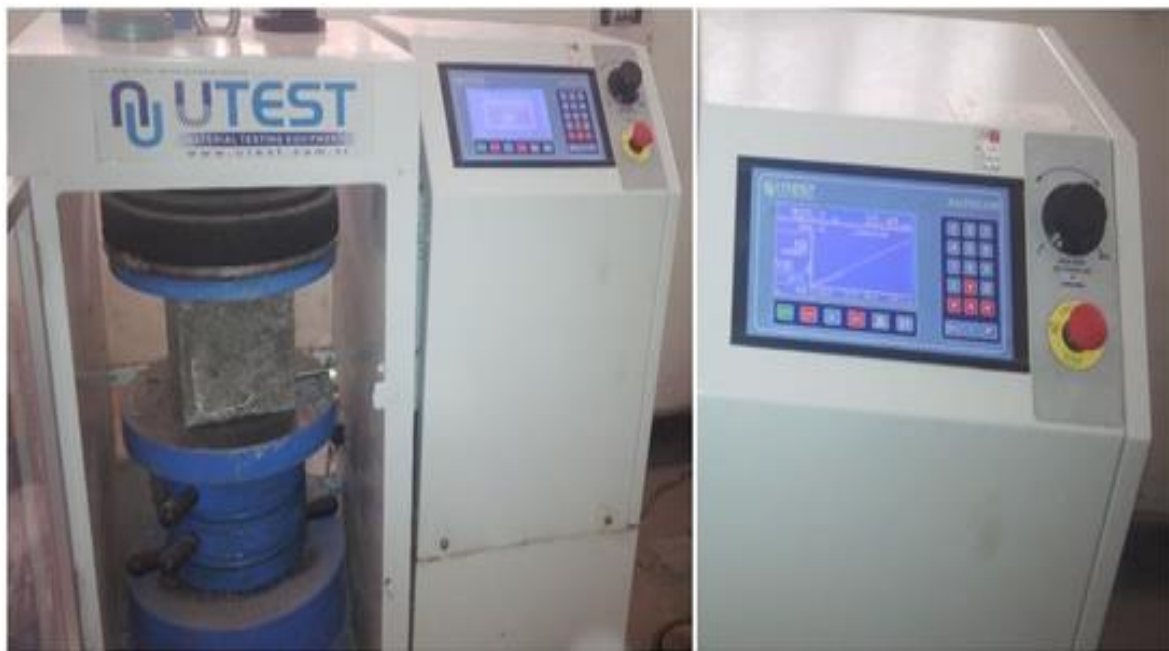
Fig 2:- Concrete Cube Testing
