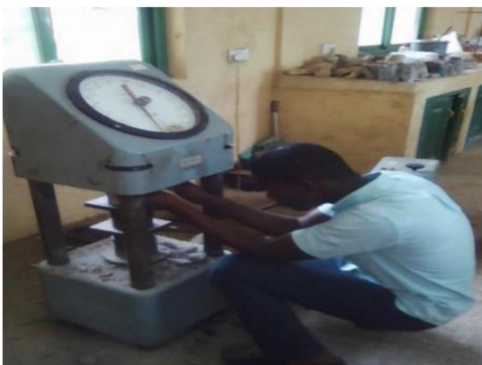
Fig 3a: compressive test machine in use
