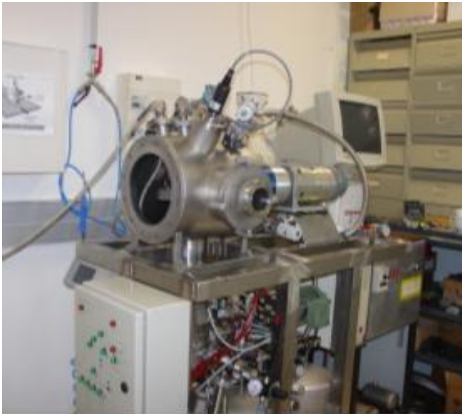
Fig 1:- The general view of tribometer pion-disc type (disc support, chamber, vacuum pump)
