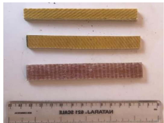
Fig.2:- Specimen for Flexural Test
