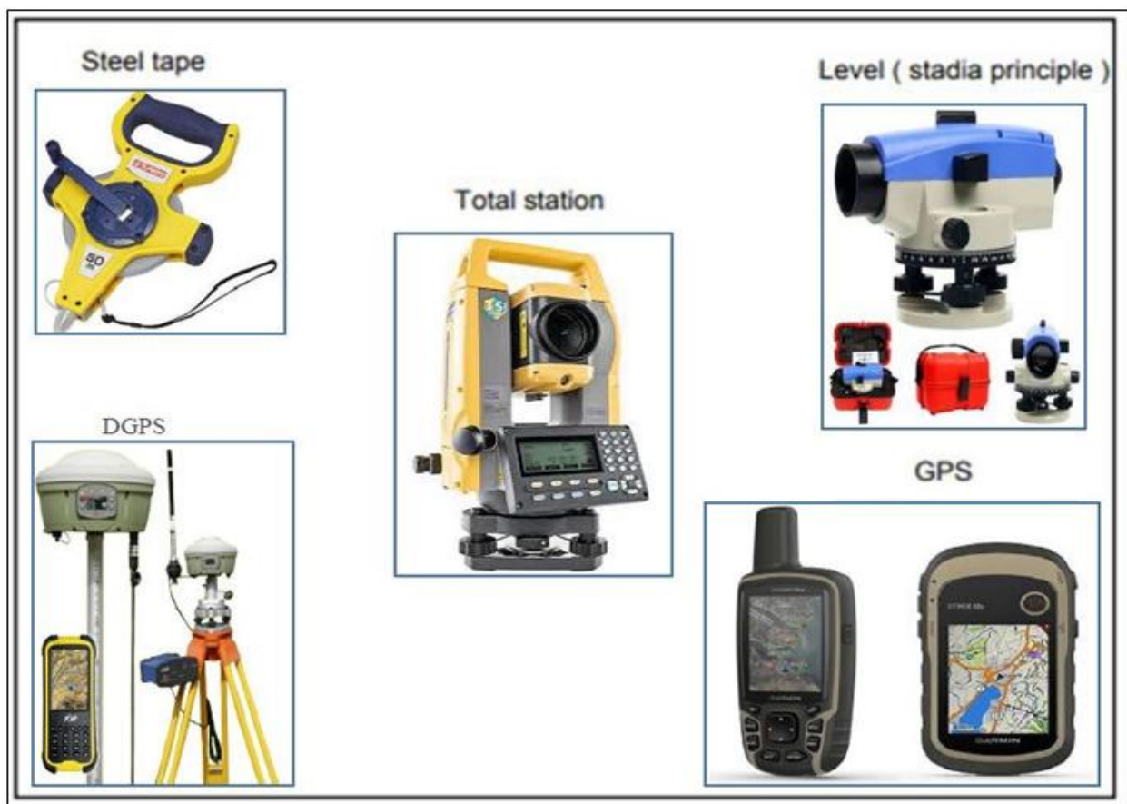
Figure 1:- Tools and materials in land surveying
