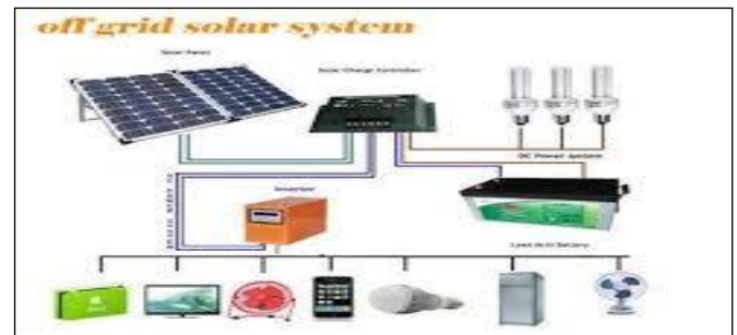
Figure 1: Typical solar home systems configuration diagram, Source: [9]
