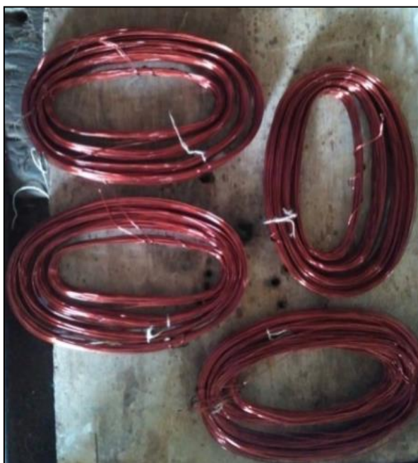
Fig 4:- Running coils of Single phase winding
