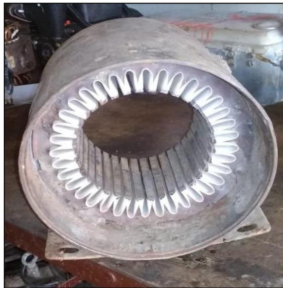
Fig 2:- Empty stator core and casing
