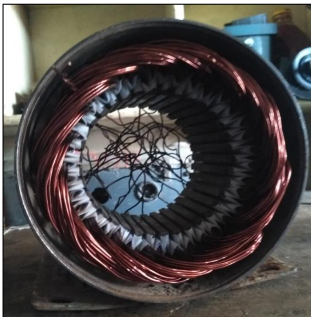
Fig 3:- Three Phase winding insertion
