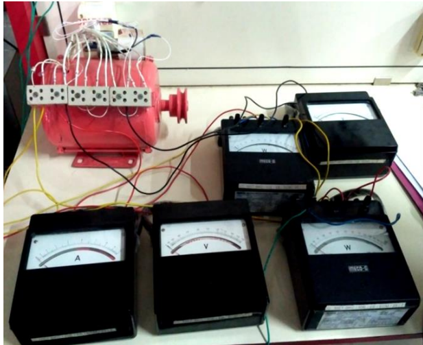
Fig 7:- Three Phase No load and block rotor test setup
