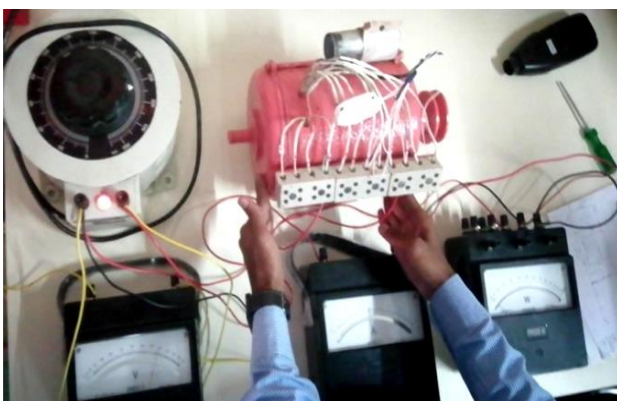
Fig 8:- Single Phase No load and block rotor test setup
