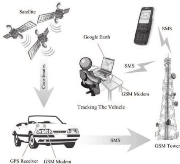
Fig 2:- Vehicle Tracking and Anti-Theft System
