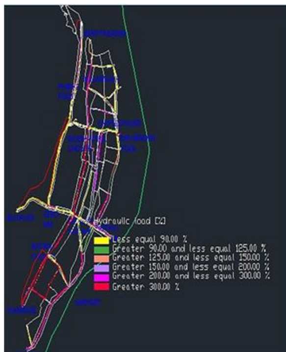
Fig 3:- Grade of Hydraulic Load of the Drainage Conduit in Existing Condition (Source: Basnet et. al, 2020)
