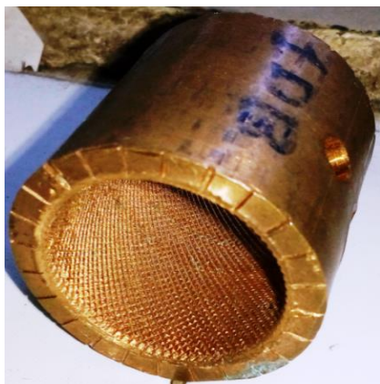
Fig. 1. Surface texture bearing of diamond shape.
