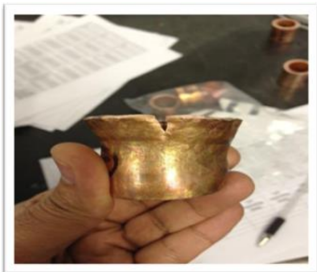
Fig 2 (b) Specimen after fracture
