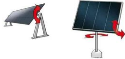
Fig 3:- Types of solar tracker
