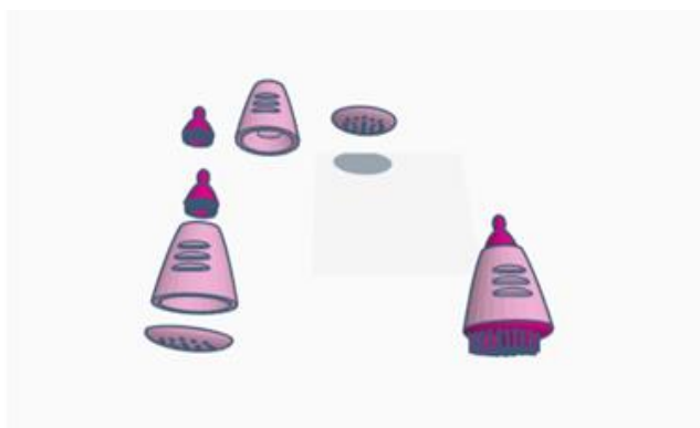
Fig 3:- 3D model of the loofah; the 3 parts and the overall design
