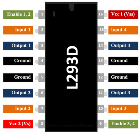
Fig 7. Pin Description of L293D
