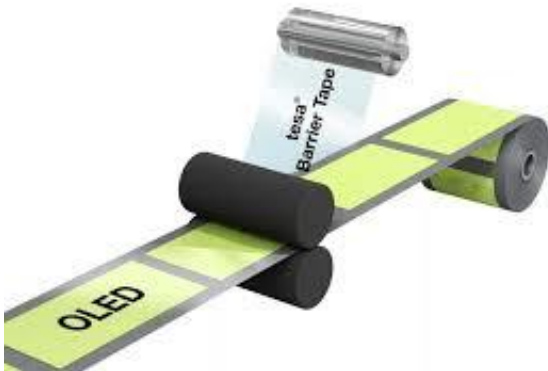
Fig 9:- Flexible OLED produced using R2R printing.
