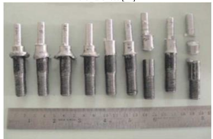
Fig 12:- Friction welded AISI 1030/AA6063-6SiC-3Gr joint [11]
