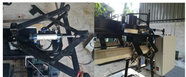
Fig 4:- Clamping Unit and Carrier Unit of the Prototype Left: Clamping Unit Right: Carrier Unit
