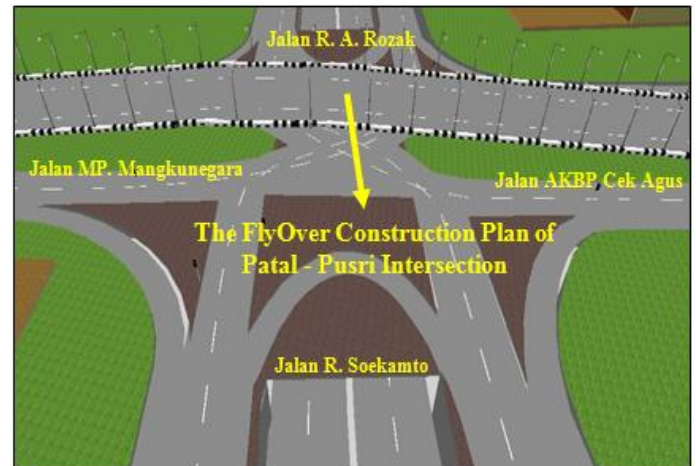
Fig 5:- The forth scenarios alternative, Flyover Construction and Geometric Changes on the Intersection’s Leg Crossing
