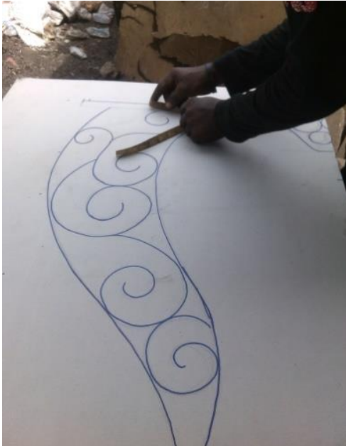
Fig 10:- measuring the design area for cutting.
