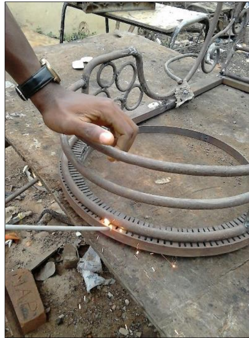
Fig 16:- joining by welding the members together
