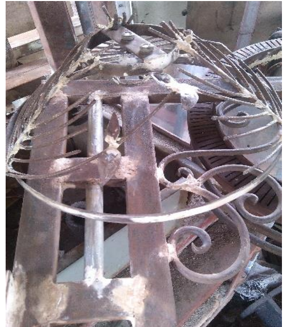
Fig 21:- Auto filler filled and sanded surfaces
