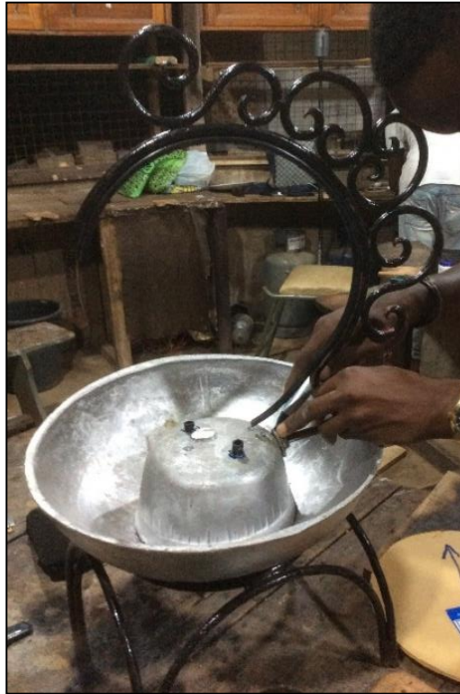
Fig 21:- connection of the frame to the basin
