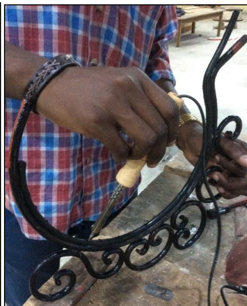
Fig 18:- Creating holes for water passage.
