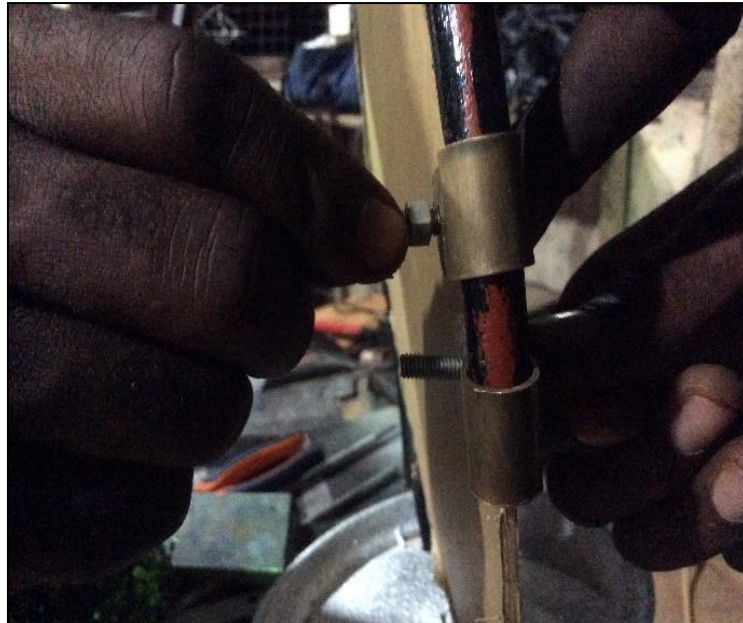
Fig 23:- connecting the frame and the fiber grass together using the brass pegs
