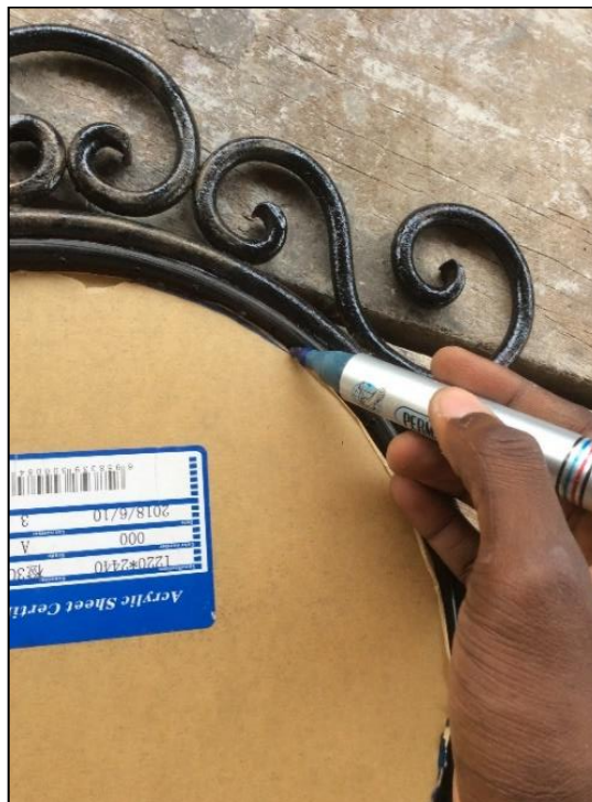
Fig 22:- Marking the fiber glass according to the frame.
