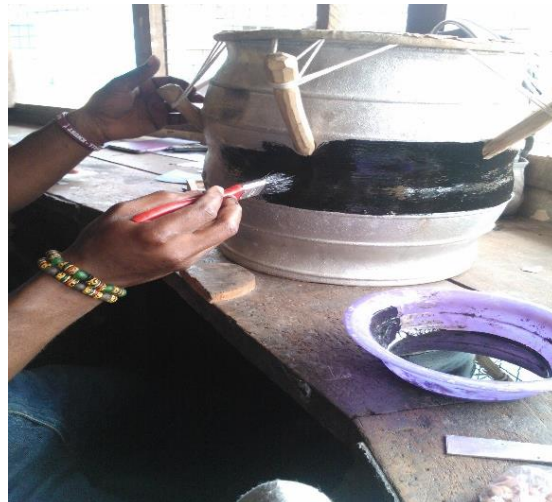
Fig 22:- middle belt of the drum being painted with oil based paint for decoration
