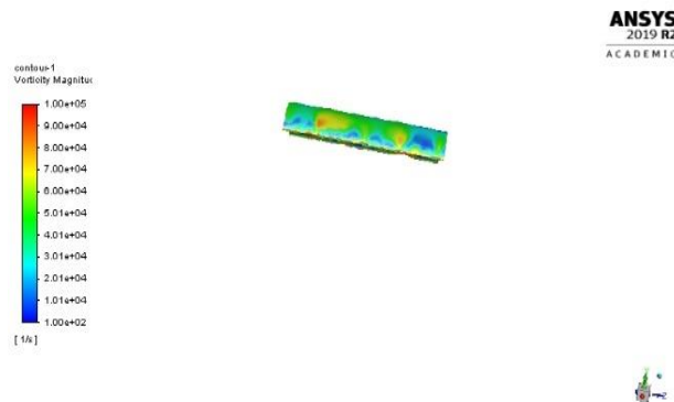
Fig 14:- vorticity contour of Basic blade at leading edge
