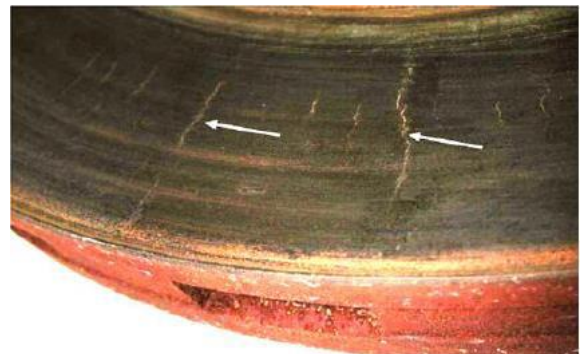
Fig 1:- Thermal cracking in disc brakes.
