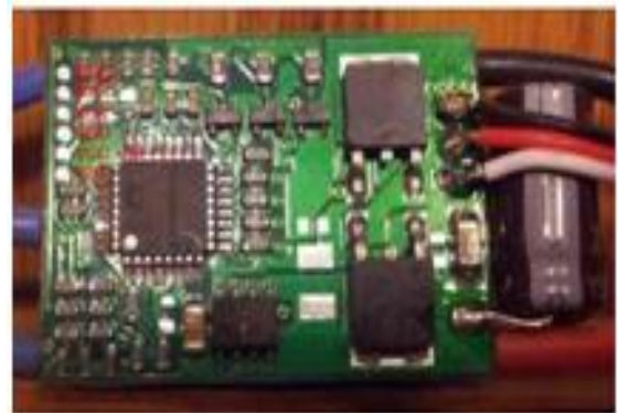
Fig 3:- Internal Circuit of Electronic Speed controller
