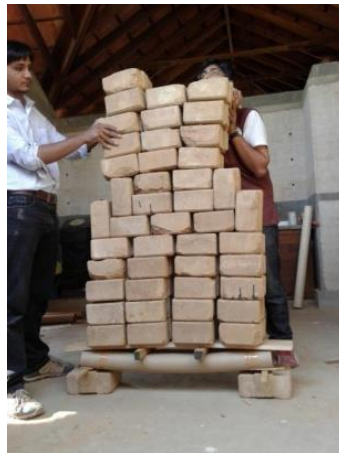
Fig 4:- Load testing of Paper tubes
