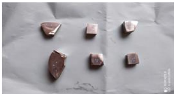
Fig 6:- Aluminum -Zinc Alloy of As Cast & Centrifugal Casting Specimens trails for Brinell hardness test
