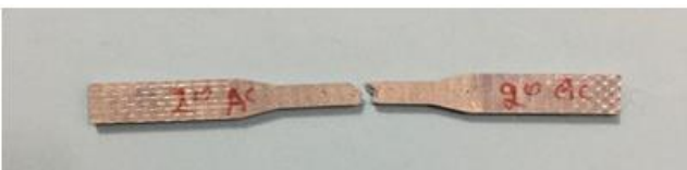
Fig 15:- Al-20% Zn as Casting
