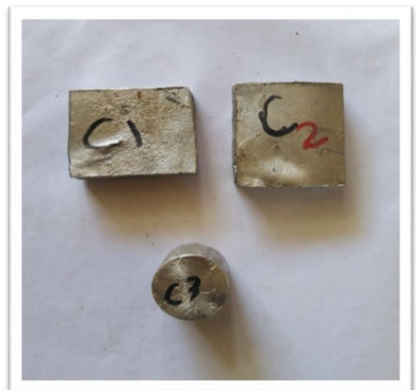
Fig 9:- specimen for compression test
