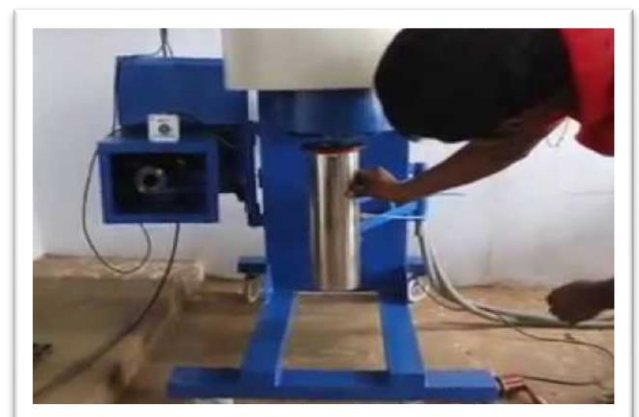
Fig 5:- Pouring of molten Al into mould
