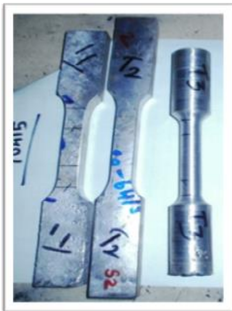
Fig 7:- Specimen for tensile test
