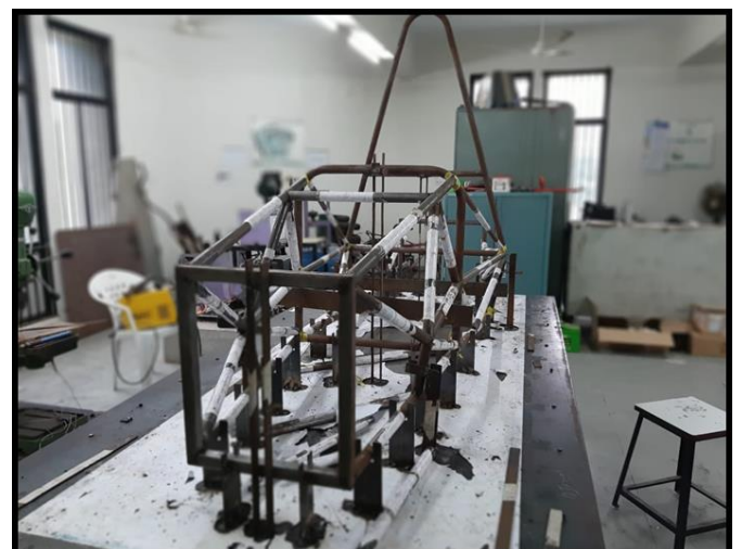
Fig. – V.H.1 (Final Set up on fixture table)
