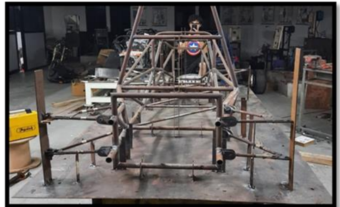
Fig. – V.G.1 (Prototype uprights as jigs)
