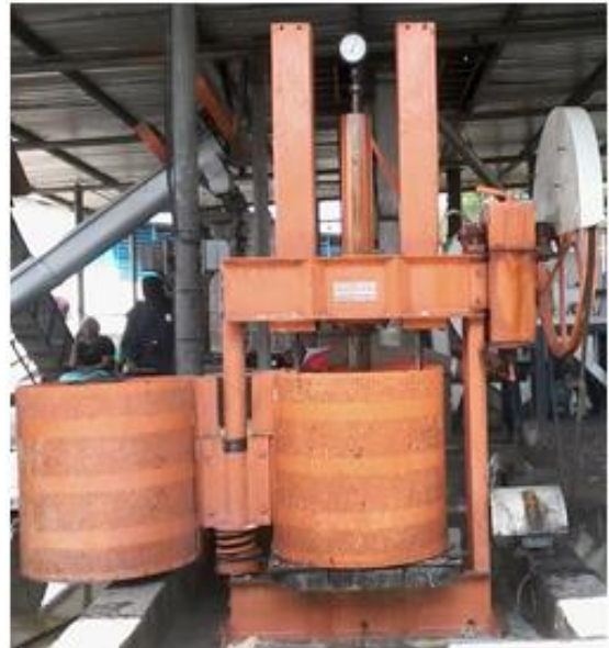
Fig. 6b: Electrical Dewatering Machine (2000kg/hr)
