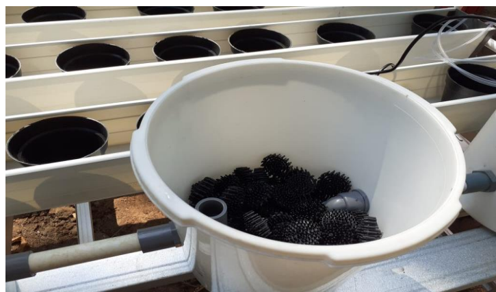
Fig 2:- Filter basket containing jagged rubber balls
