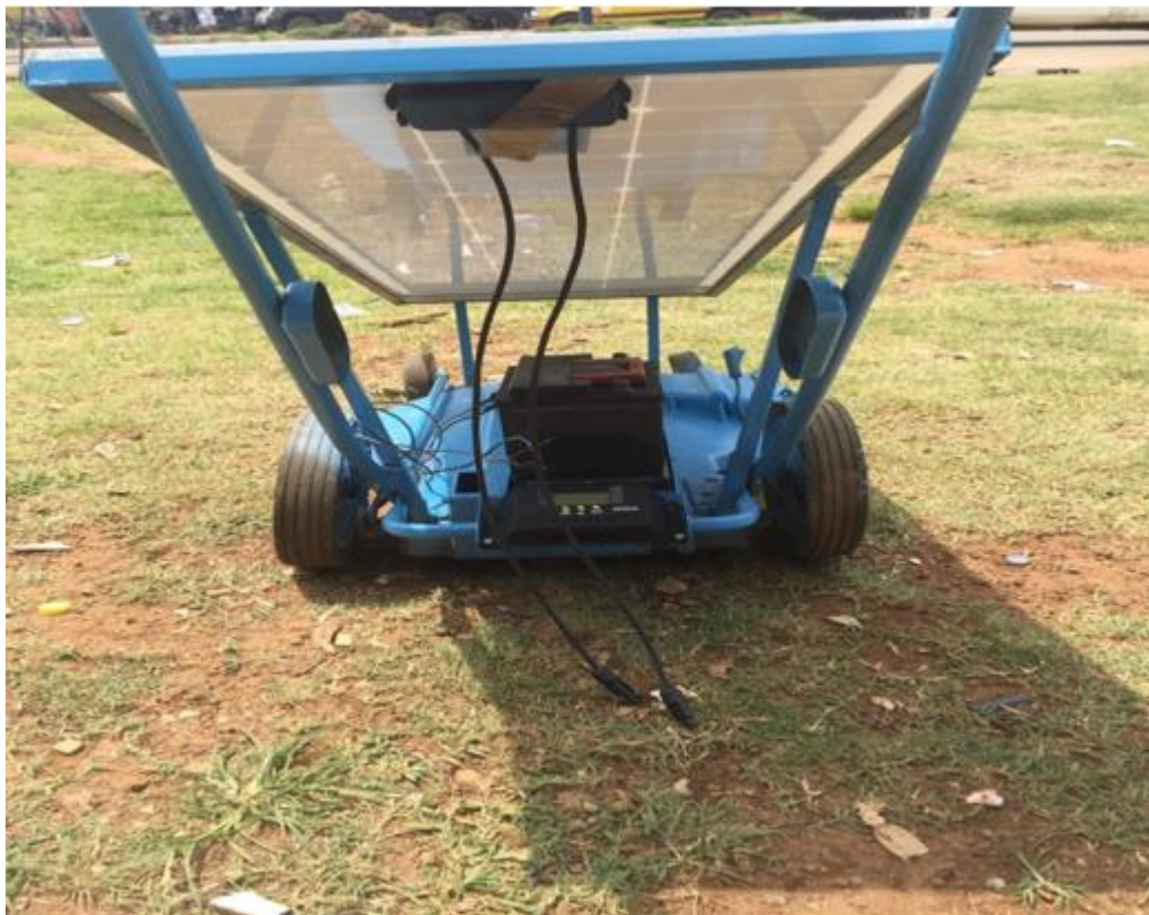
Fig 4.3: Back-view of the solar lawn mower showing the battery and charge controller.
