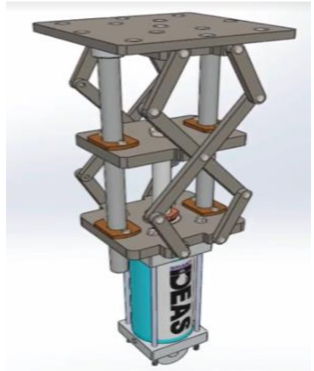
Fig 4: shows High Power Capacity Electrical Actuator which replaces the conventional manual method of handle driven plunger in GOAB switch.
