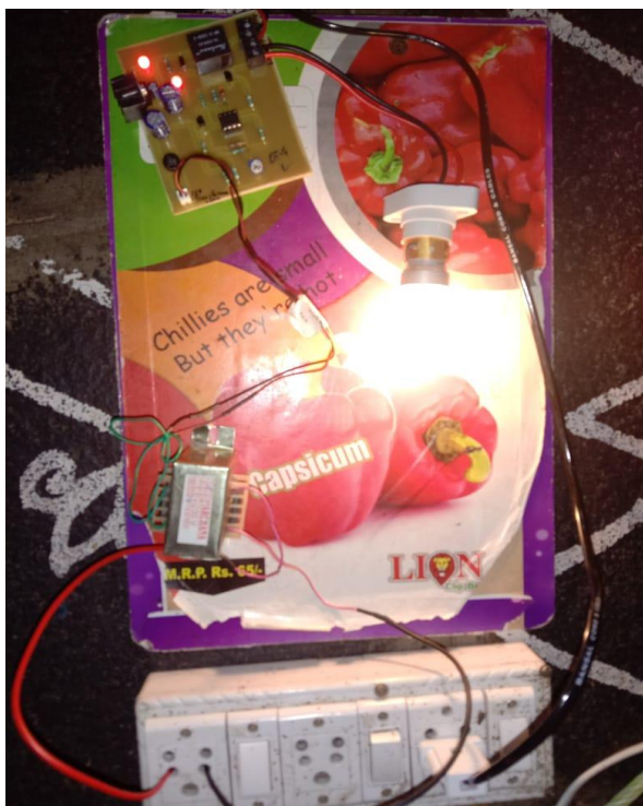
Fig.10. Proposed System when there is no over voltage and under voltage in AC supply mains
