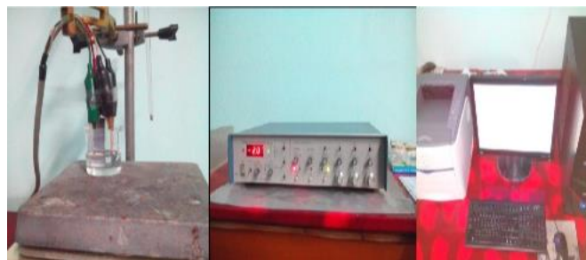
Fig. 1 The instrumental set-up of the three electrodes cell connected with the potentiostat/galvanostat via transducer with winDaq software installed computer system
