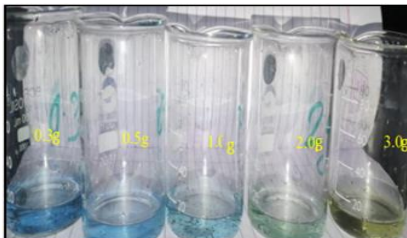
Fig 6:- Effect of addition of different amount of guava leaf powder on dye adsorption
