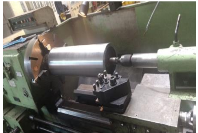
Fig 4- Turning & facing operation
