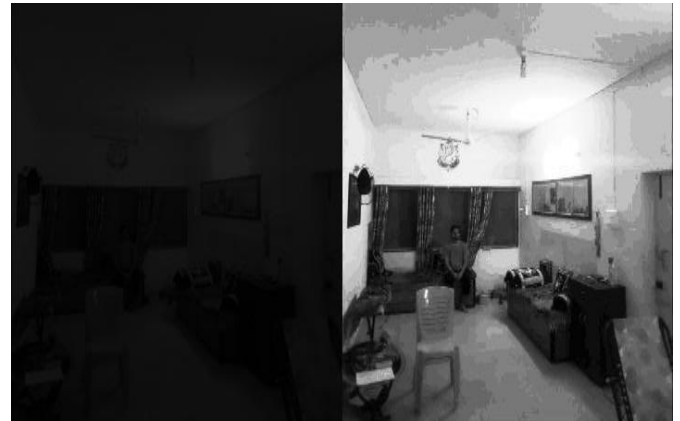
Fig. 2e. Side-by-side comparison of the initially captured image and the resultant image after applying histogram equalization.
