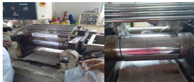
Fig. 1: Mastication operation of Two Roll Mixing Mill
