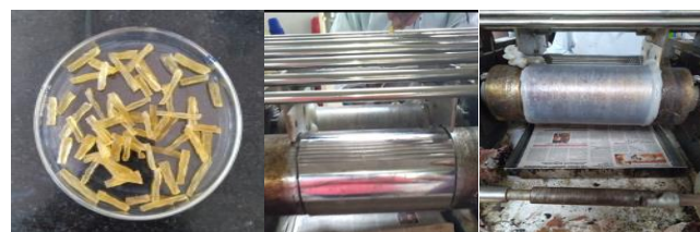
Fig. 2: Addition of natural rubber into polyethylene matrix
