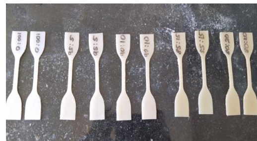
Fig. 8: Test specimen for Tensile Test
