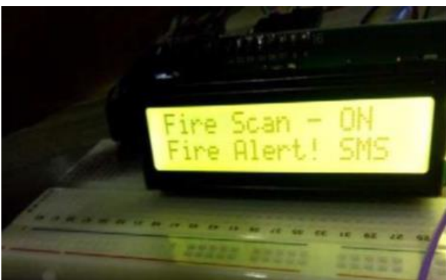
Figure 8: When the thermistor based temperature sensor detects fire and a notification message appeared on the LCD display
