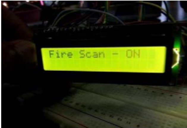
Figure 6: When the thermistor based temperature sensor is in ready mode to detect fire.
