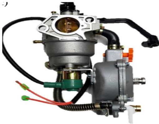
Fig 2:- Diagram of dual carburetor for LPG and Gasoline (14).
