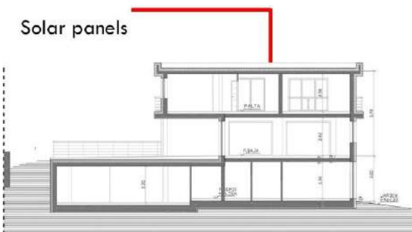
Figure 11.7 The position of the Solar panels on top of the roof surface
