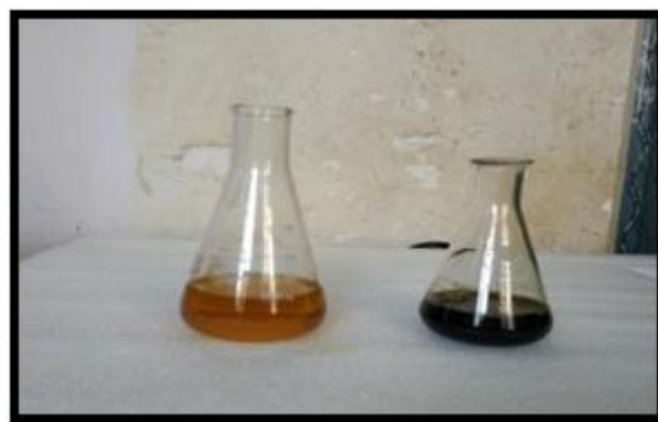
Fig: 2 (i)Plant Extract, (ii)Colloidal solution of NPs
