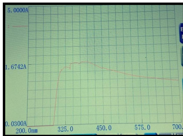
Fig: 6 UV-Visible Spectrum of Malachite Green after degradation
