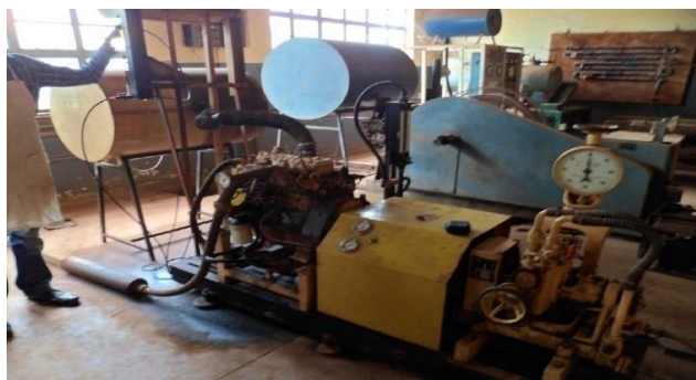
Plate 1: Perkin 4:108 diesel engine mounted on Steady state engine test bed at UNN Nsuka
