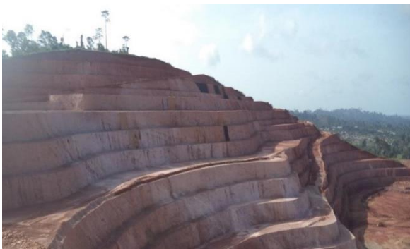
Figure 2: A quarry showing staged ore extraction (saprolite ramps)
