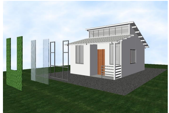
Fig. 2. Extrusion of elements that composes the façade with architectural envelope with water containers.
