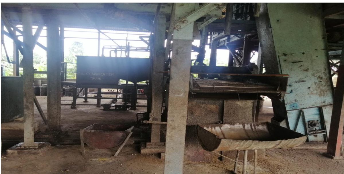
Plate 3: Palm fruits Heater and Processor Machine that is connected to the Clarification Tank
